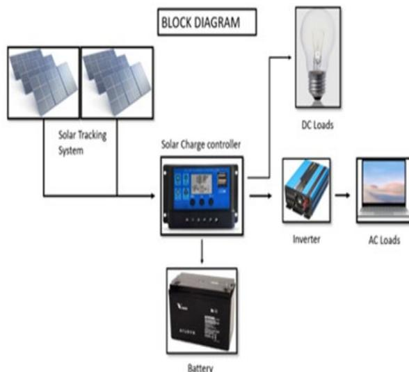
Figure 5: Block Diagram
