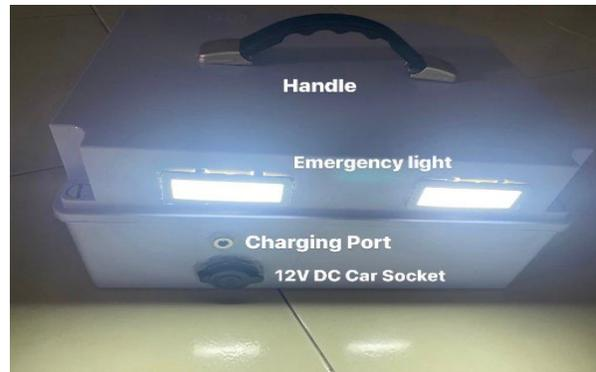
Figure 14: Portable Solar Generator Front View
