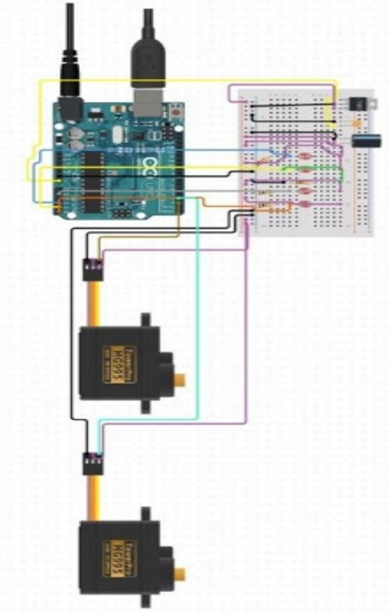
Figure 6: Circuit Diagram for Dual Axis Solar Tracker
