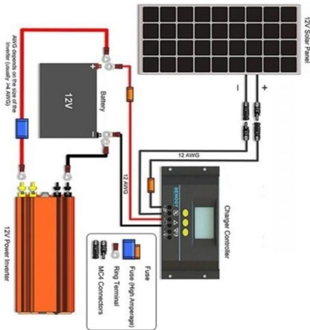
Figure 7: Circuit Diagram for Portable Solar Generator
