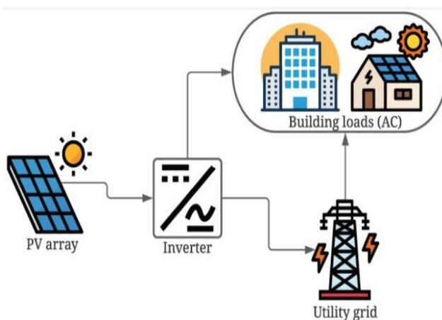
Figure 4: Grid-Connected Solar Generation System
