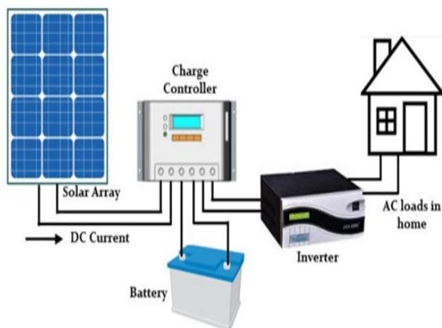
Figure 3: Off-Grid Solar Generation System
