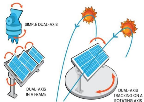
Figure 2: Dual-Axis Solar Tracker
