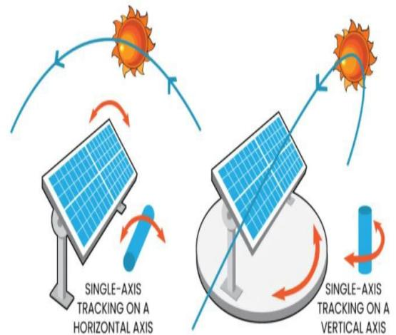
Figure 1: Single-Axis Solar Tracker
