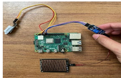
Figure 9: Installation of Raindrop Sensor
