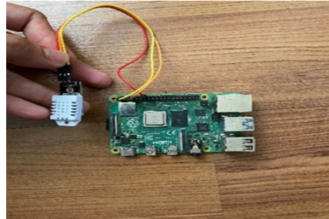
Figure 8: Installation of DHT22 Sensor
