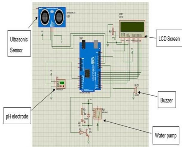
Figure 9: Circuit Diagram of the designed system
