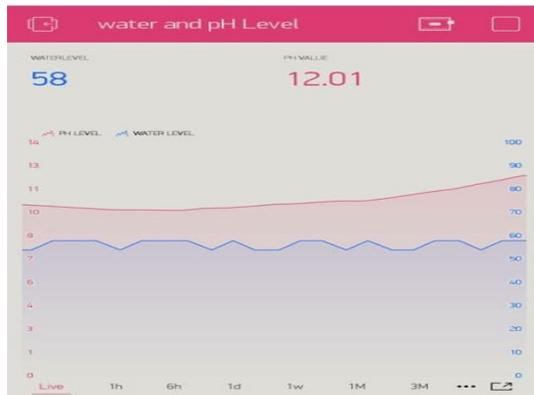
Figure 13: Reading from Blynk Apps for Alkaline Solution
