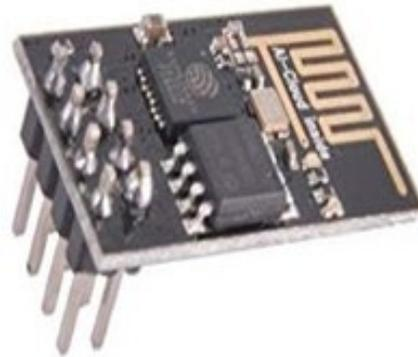
Figure 6: ESP8266 module
