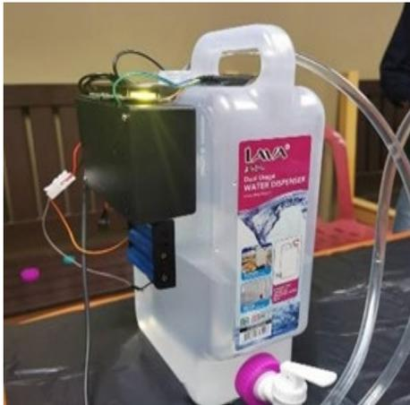
Figure 10: Dual sensors device for pH and Level Measurement
