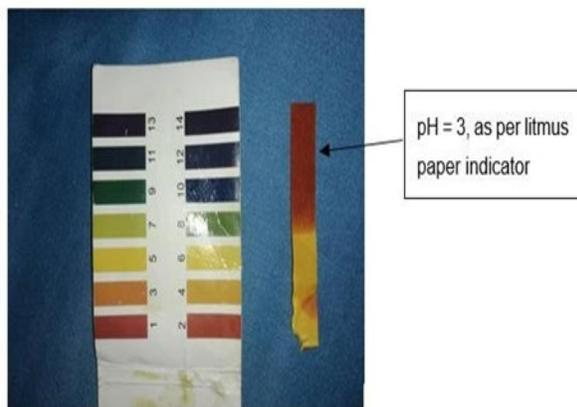
Figure 14: pH Litmus paper for the Acid Solution
