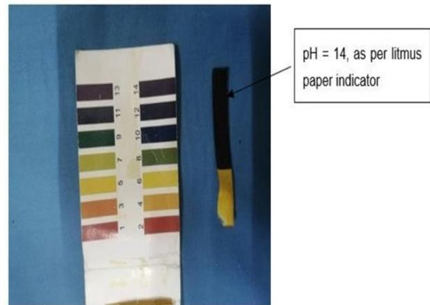
Figure 16: pH Litmus paper for Alkaline Solution
