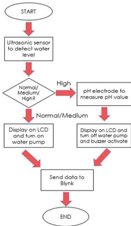
Figure 8: Flow chart of the designed system
