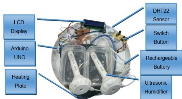
Figure 4: Hardware Placement inside the casing.
