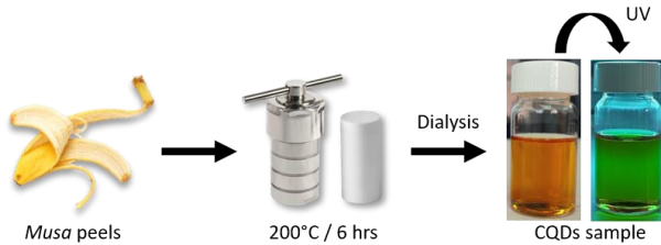
Fig. 1: Hydrothermal synthesis of CQDs sample
