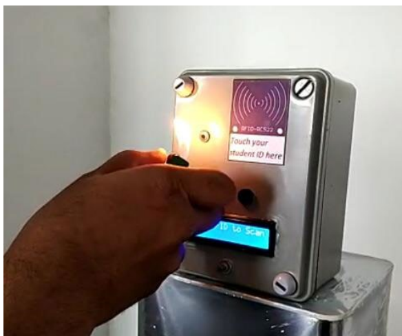
Figure 7 Testing on temperature sensor by using lighter
