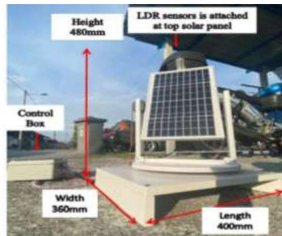
Figure 6: proposed dual axis solar tracker prototype
