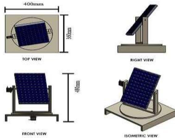
Figure 5: 3D design of the proposed solar axis tracker; the front view, isometric view, and top view
