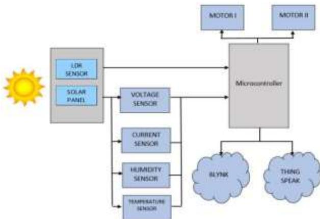
Figure 1: The proposed dual axis solar tracker with IoT monitoring system
