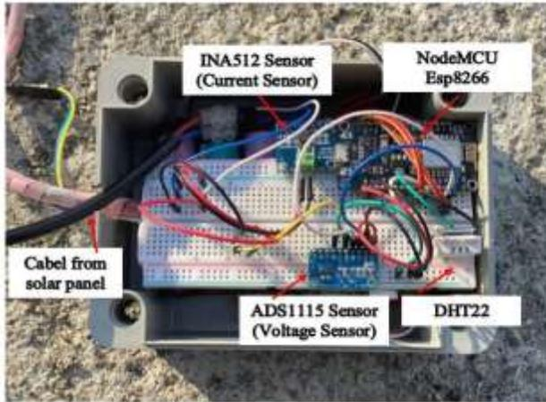
Figure 8: Electrical wiring of sensors
