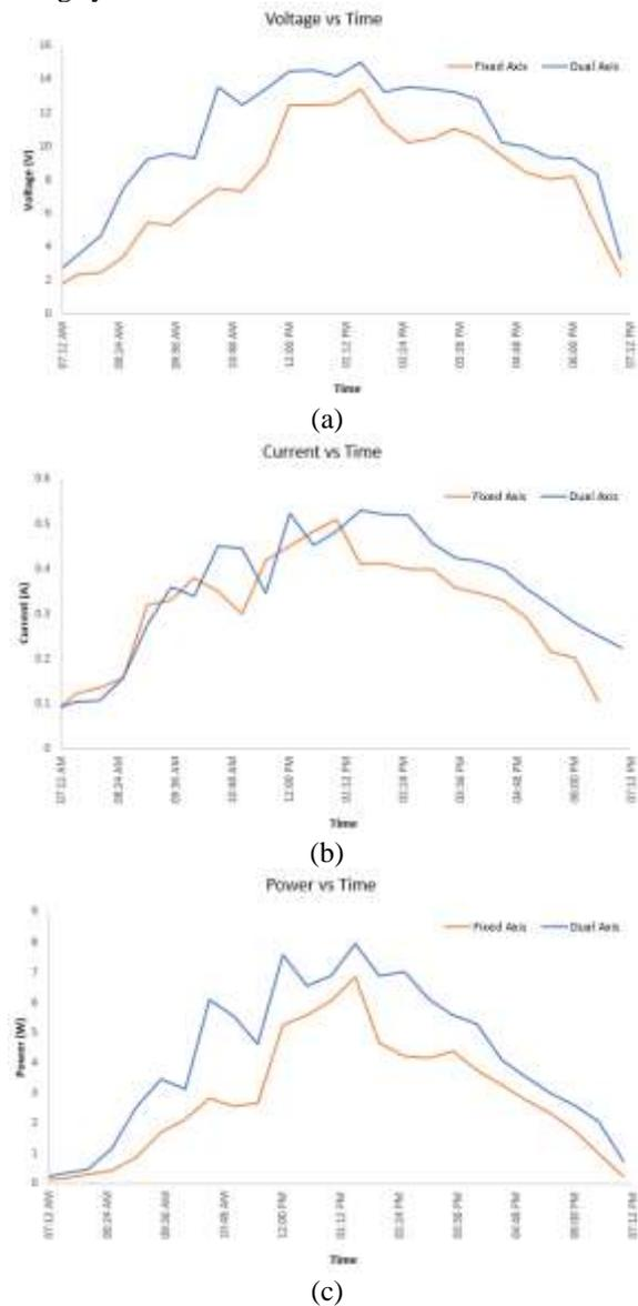
Figure 14: shows the measured parameter results (a) voltage, (b) current and (c) power of dual axis solar tracker recorded at 7.00am to 7.00pm.
