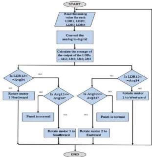
Figure 2: Process of dual axis solar tracking
