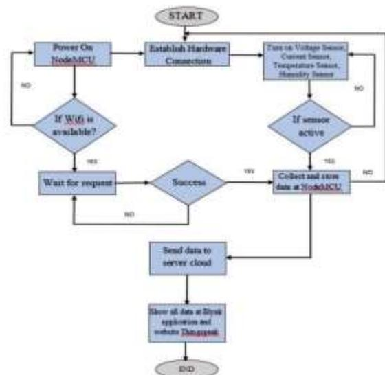
Figure 3. Process of IoT monitoring
