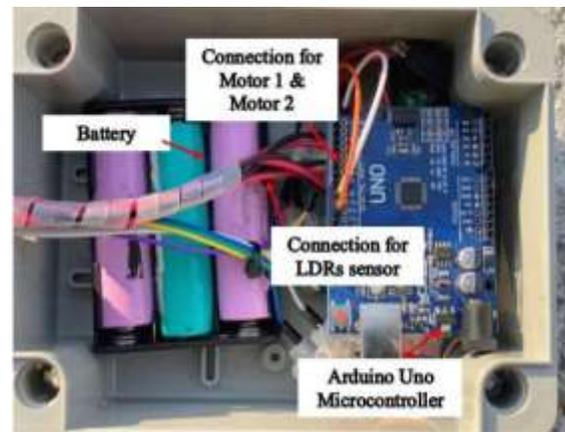
Figure 7: electrical wiring of controller
