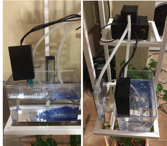
Figure 4: The prototype of Aquarium Monitoring System.
