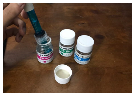
Figure 2: Calibrating pH sensor using 3 buffer solution.
