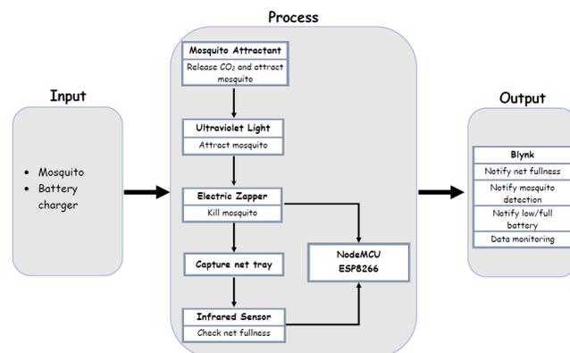
Figure 1: Block Diagram for the entire project.
