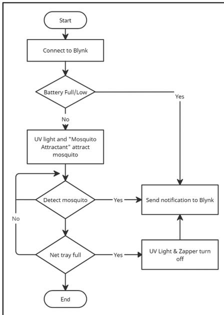
Figure 2: Flowchart Diagram.
