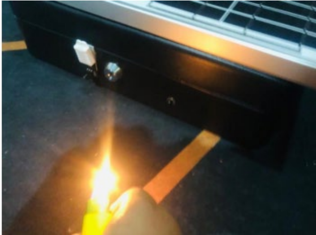
Figure 4.5: Flame sensor demonstration
