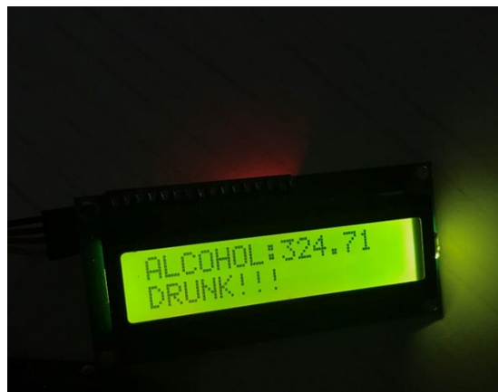
FIGURE 3. The alcohol level is between 300 to 400 for 'DRUNK!!!' condition.
