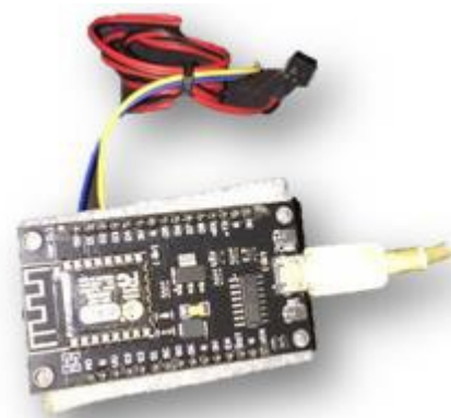
Figure 7: NodeMCU connection with Push Button
