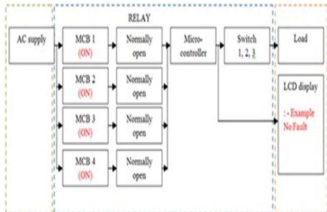
Figure 5: Process flow block diagram before MCB tripping
