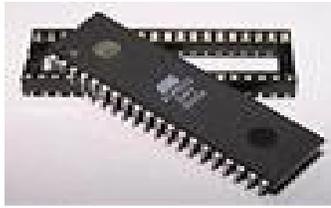
Figure 1: Microcontroller 80C51
