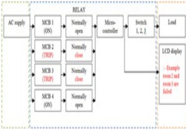
Figure 6: Process flow block diagram after MCB tripping
