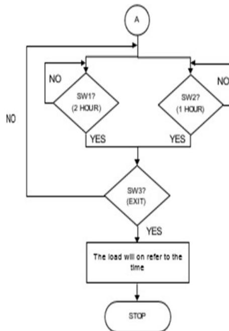
Figure 8: Flow Chart of Power Saving Device
