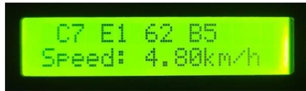
Figure 4.3: LCD displaying the UID and Speed of the Vehicle.
