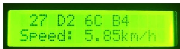
Figure 4.4: LCD displaying the Speed and the UID of the Vehicle.
