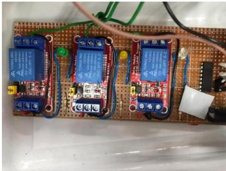
Figure 6: Relay and Relay Driver circuit that has been constructed
