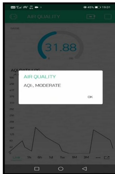
Figure 8: Notification display given when the gas density increases according to the gas level
