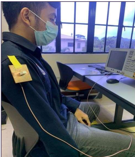
Figure 4.5: Validate the fabricated antenna on human body
