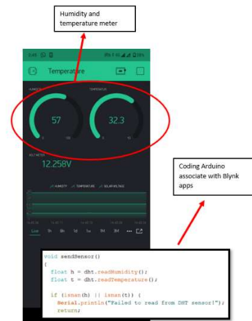
Figure 4.3b: Humidity and temperature meter Blynk interface indication
